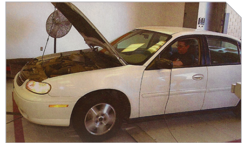
K&N technician Dave Davey began by running our 2005 Malibu Classic on a SuperFlow chassis dyno to establish the baseline horsepower and coolant temperature numbers.
