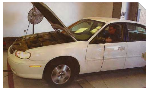
K&N technician Dave Davey began by running our 2005 Malibu Classic on a SuperFlow chassis dyno to establish the baseline horsepower and coolant temperature numbers.
