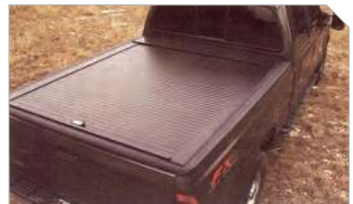
This American Roll cover was installed at Truck Covers USA. The resulting improved aerodynamics gave us another 1.56 mpg.
