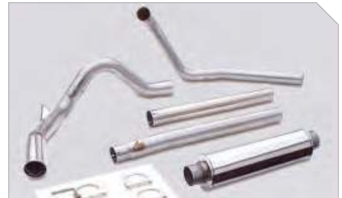
Our second test was to install a Magnaflow turbo back exhaust system. Mileage increased by just seven tenths of a percent, but power increased by 6.2 percent.
