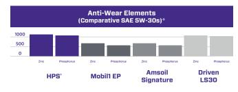
Anti-wear additives are used to prevent metal-to-metal contact in areas where achieving a full fluid film of oil is not possible either due to excessive load or engine design. The camshaft(s) and lifters as well as piston skirts are key examples of areas relying heavily upon anti-wear metals. Performance engines, particularly, need higher quality and increased amounts of antiwear additives due to greater loads on the camshaft caused by higher ramp rate camshafts and higher springs pressures.
