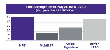
Film strength is the oil's ability to withstand a load without being displaced by pressure. Film strength is very important in areas designed to have full hydrodynamic lubrication (HDL) such as the crankshaft and rod/ main bearings. A lack of film strength leads to greater metal-to-metal contact and wear throughout the engine. High film strength is key in performance engines and/or forced induction engines which see more severe operation and a higher rate of crank flex.
