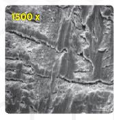
The bearing is scuffed after using a leading synthetic motor oil.
