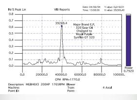
200 HP Roots Blower at a chemical plant is experiencing high vibrations while being lubricated with a competitor's ISO 320 EP gear oil.
